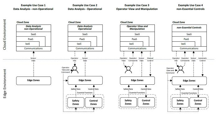
Figure 1 – Example Use Cases – Zone and Conduit Partitioning
