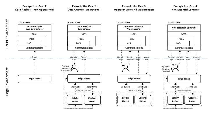
*Figure A.4 – Example Use Cases – Zone and Conduit Partitioning*
